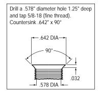
Figure 3. Drill and Tap Detail
