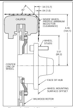
Figure 2. Wheel Clearance Diagram
