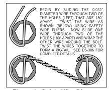
Figure 4. Safety Wire Diagram
